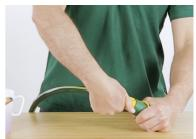
The **Hose Connector with Flow Control** is designed to be used at the spray end of the hose. Water must flow through and out of this connector. This connector will leak if water flow is directed the wrong way.
